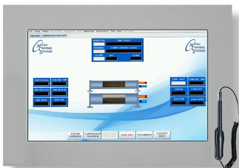
EVAPORATOR CONDENSER OVERVIEW SCREEN
